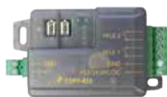
COPY-433 2-channels 433,92 MHz receiver dimensions 77x42x18 mm
